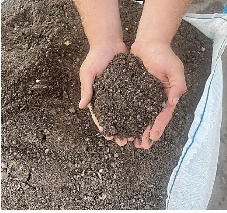
Rasengittersubstrat Körnung des Substrates 0–12mm
